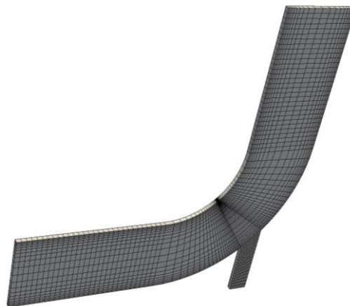
Figure 1.1 The Hex Fine mesh created using GAMBIT
